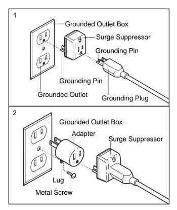
The temporary adapter should be used only until a properly grounded outlet (drawing 1) can be installed by a qualified electrician.
